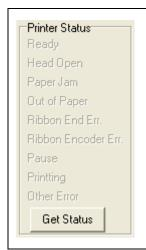
When connecting printer with USB or RS-232 interface, the "Get Status" button will be visible to polling printer status.
